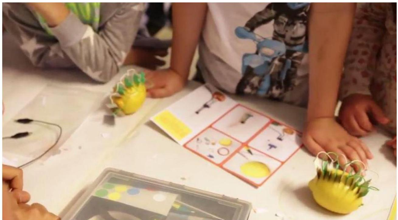
Constructing a battery solely out of lemons (voltaic elements). The kids will experience the making of a battery with one or two lemons, using it to light up a LED lamp. The circuit presented is one of the classic school experiments, with one twist: in the circuit, an 'energy thief' will be added, else known as «joulethief.»
