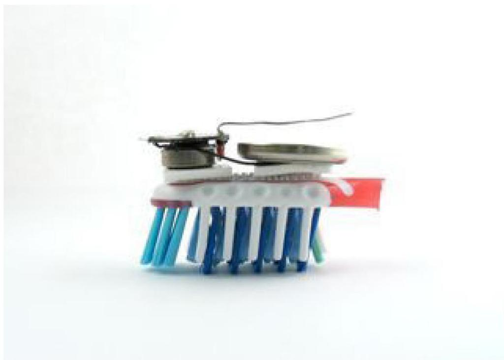
In this technological experiment, the kids have the chance to build their very own micro-robot out of a toothbrush. They will be introduced to the way of transmitting movements through small vibrations as well as how to make the robots move towards the same direction.
